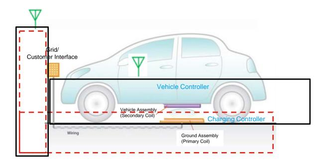
UL 2750: Verification of Wireless Charging Base Safety (Draft) <- MOU -> SAE TIR J2954: Wireless Power Transfer and Alignment
